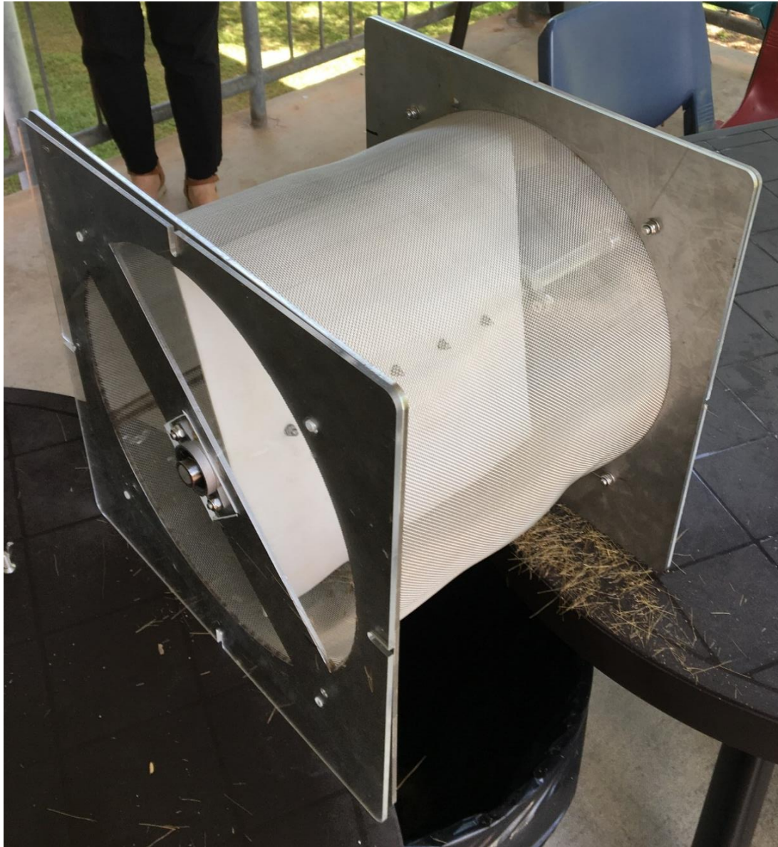
Figure 2: Mark 3 showing base plate arrangement. Note deformed mesh.
