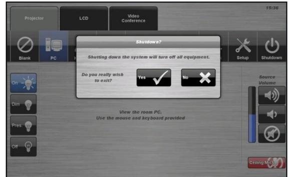
**NOTE:** Letting the system go to sleep by itself only powers down the touch panel screen, it **does not turn off** the audio-visual equipment. To turn off the equipment, shutdown the system properly using the touch screen panel. This will extend the life of the audio-visual equipment.
