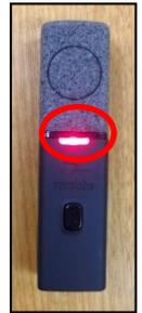
**To turn on** -> Remove from charging dock and wait for 3 seconds, until the LED flashes red. Press the button on the front of the microphone to activate. The LED lights will flash green every few seconds to show that the microphones are active.
