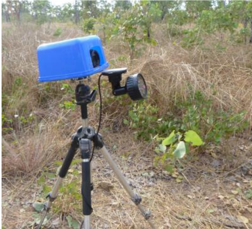
Figure 8 Set-up of an infra-red lamp directly underneath the video camera on a tripod, and showing one approach for water-proofing the camera. Note that the 12 V battery to which the infra-red lamp is attached is underneath the tripod but not photographed in this instance.
