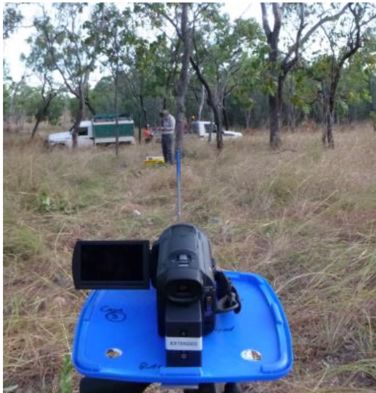
Figure 9 Behind-camera view of the vertical alignment that is to be instated from the video camera to the fence dropper and through to the reference tree (noting that, in this photograph, the speaker is not yet attached to the fence dropper).
